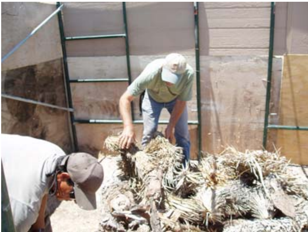
Seen here are Oscar Mora and Greg Seymour arranging the fuel around the pots prior to firing. The wood wall in the background is to help contain the fire—a wise precaution for the summer 2005 fire season.
