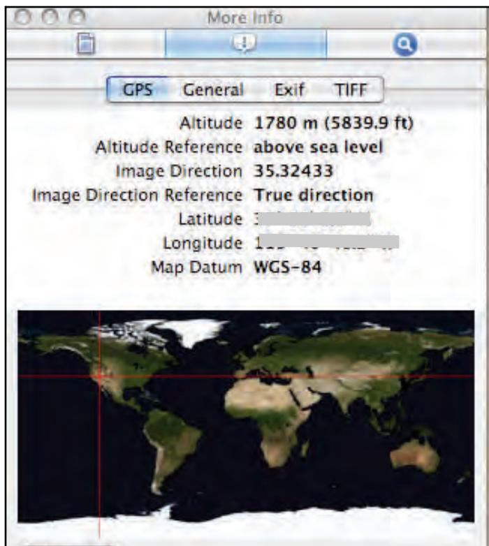
The data (UTM's or Lat/Lon) are set as preferences by the user in the “preferences options” in the Theodolite Application. When selecting the photo, the figure on the left is brought up where you can check the (Locate) button which will reveal the position in Google Earth as pictured below.
